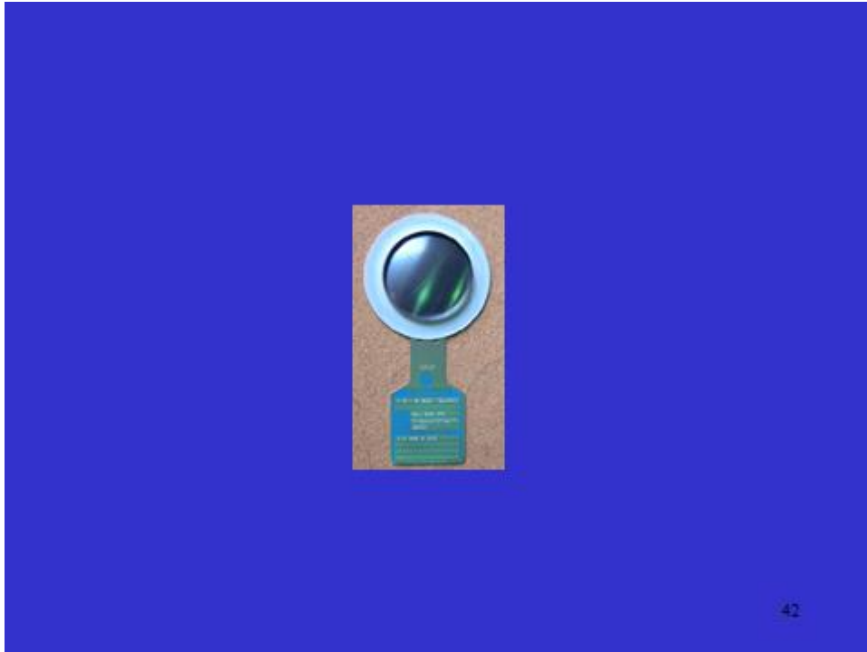
This is the sort of bursting disc the question was about with an external diameter of about 11 cm.
