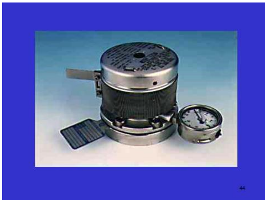
This is how it would look fitted beneath a pressure relief valve. A ‘tell-tale’ manometer (pressure gauge) is then fitted above the bursting disc and below the relief valve to detect rupture of the disc. The pressure relief valve, incidentally, is surrounded by a gauze, a flame trap to ‘prevent the immediate passage of a flame’ into a tank shell.
